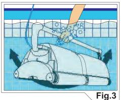
(5) To start the Commercial Pool Cleaner, press the Power Supply ON/OFF switch to the On position. If your Power Supply is equipped with an adjustable Timer (pg.6, fig 2) you can now select the length of the cleaning cycle and press the Reset button to start the cleaner. Commercial Pool Cleaner
